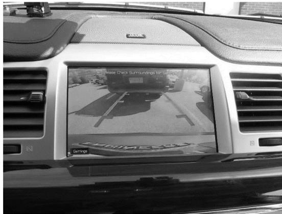
Fig. 1. Rearview camera image in the center console display.
