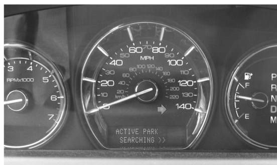
Fig. 2. Two-line text display with Active Park Assist system status and instructions.
