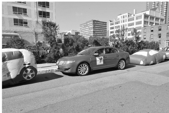
Fig. 3. Study vehicle parallel parked between two inflatable cars.
